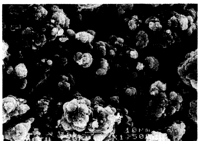
Figure 4 Scanning electron micrographs of PA/PPy/SDS solution side: a , without enzyme; b , with enzyme entrapped in the matrix.
