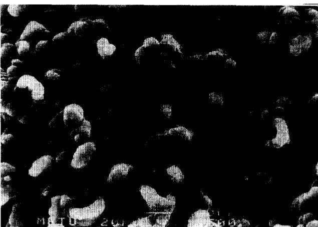
Figure 3 Scanning electron micrographs of PA/PPy/ClO 4 - solution side: a , without enzyme; b , with enzyme entrapped in the matrix.
