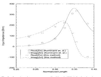
Fig. 2. Input impedance versus normalized length  $(l/\lambda_0)$  for the slot given in Fig. 1 (w/l = 0.02 cm,  $h_1 = h_2 = 0.0$  cm,  $\varepsilon_{r3} = 2.55$ , and d = 5.0 cm).
