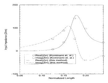
Fig. 3. Input impedance versus normalized length  $(l/\lambda_0)$  for the slot given in Fig. 1  $(w/l = 0.02 \text{ cm}, h_1 = h_2 = 0.0 \text{ cm}, \varepsilon_{r3} = 12.8$ , and d = 5.0 cm).
