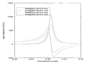
Fig. 4. Input impedance versus normalized length  $(l/\lambda_0)$  for the slot given in Fig. 1  $(w/l = 0.02 \text{ cm}, h_1 = 0.2 \text{ cm}, h_2 = 0.05 \text{ cm}, \varepsilon_{r1} = 2.55, \varepsilon_{r2} = 12.8, \varepsilon_{r3} = 1.0).$
