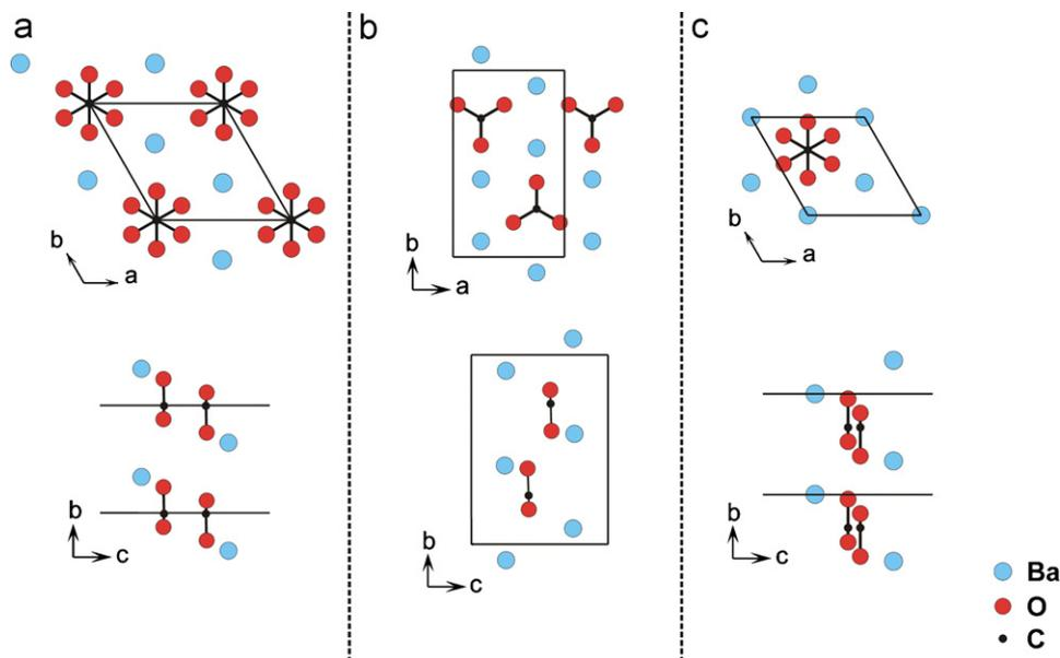
Fig. 3. View along  $[001]$  and  $[100]$  of the  $[\text{Ba}_2\text{CO}_3]$  sheets in: (a)  $\text{Ba}_6\text{Ru}_3\text{Br}_{1.54}(\text{CO}_3)_{0.23}\text{O}_{12}$  with disorder of  $\text{CO}_3$  groups; (b) witherite- $\text{BaCO}_3$  with aragonite-type structure, and (c)  $\text{BaCO}_3\text{-II}$ .
