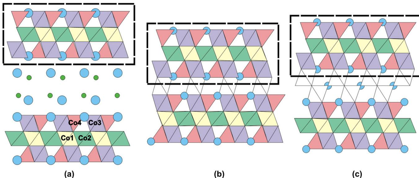
Fig. 2. View along [010] of (a)  $\text{Ba}_2\text{Co}_4\text{XO}_7$ , (b)  $\text{Ba}_2\text{Co}_9\text{O}_{14}$  and (c)  $\text{Ba}_3\text{Co}_{10}\text{O}_{17}$ . The  $(\text{Ba}_2\text{Co}_8\text{O}_{14})^{2-}$  blocks encountered in the two series are encircled with dotted lines.
