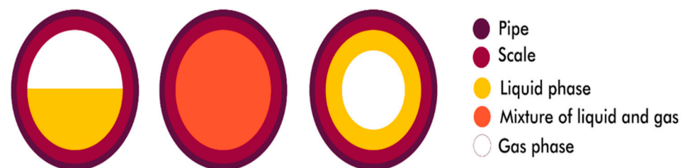
Figure 3. Simulated flow regimes from left to right: stratified, homogeneous, and annular, respectively.
