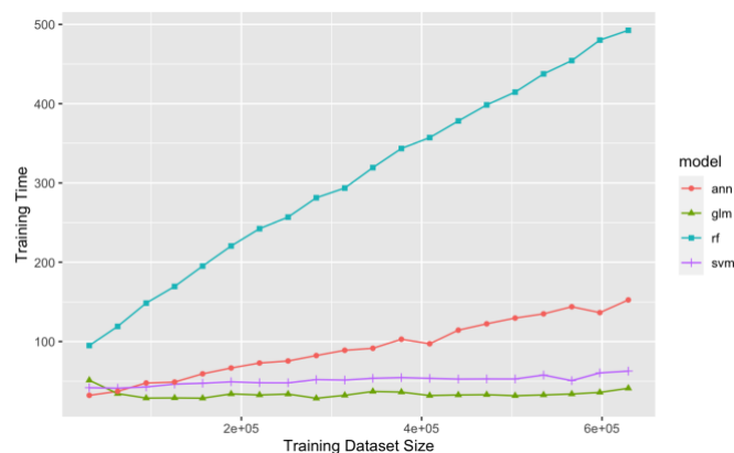
Fig. 16 Training Time in Seconds by Each Machine Learning Algorithm with Various Sample Sizes
