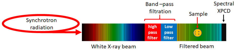
Figure 4.2: Schematic of the synchrotron setup for KES imaging. The setup considers a white beam input; a band-pass filter made by absorbers with different thicknesses and materials; and a spectral XPCD .
