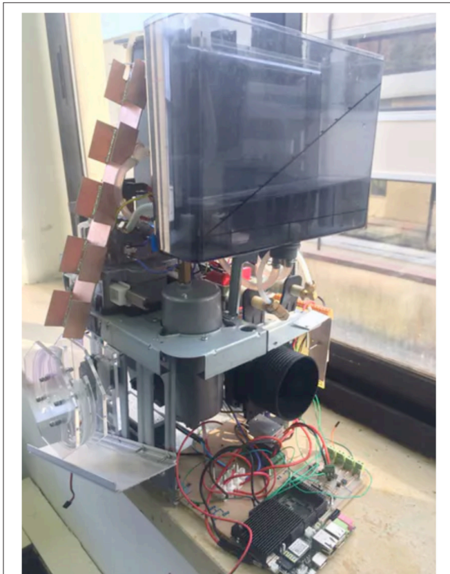
FIGURE 3 | The interactive coffee machine enabled by a UDOO Quad.
