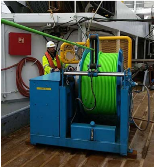
Figure 22: Tow Winch used for the CSEM Survey
