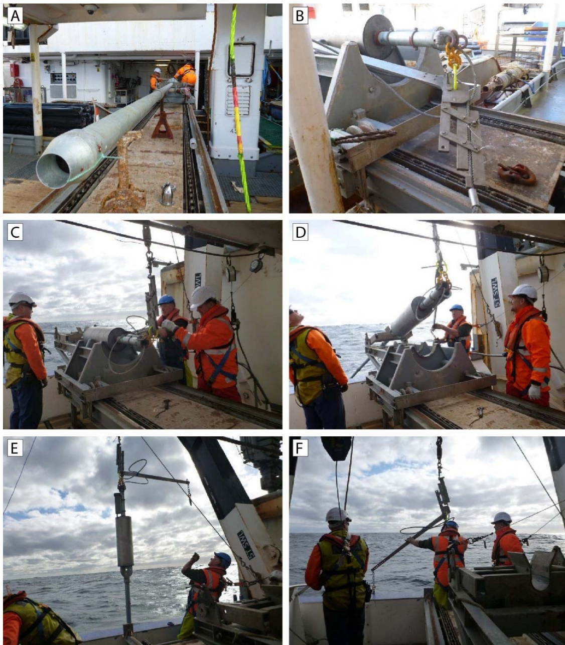
Figure 46: NIWA Piston Corer configuration and deployment procedures
