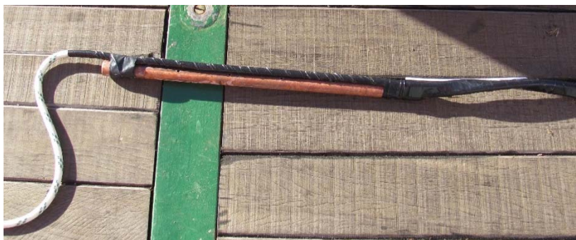
Figure 27: One of two transmitter electrodes
