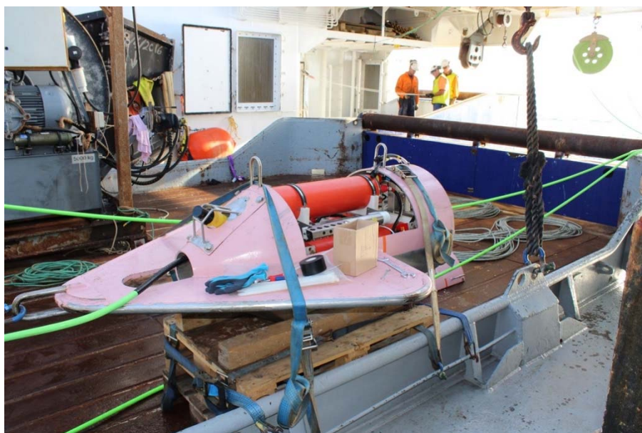
Figure 24: Pig with open lid showing transmitter pressure vessels, CTD mounted inside its body and acoustic transponder in its nose.
