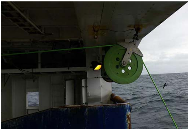
Figure 23: Block attached beneath fantail for the CSEM cable
