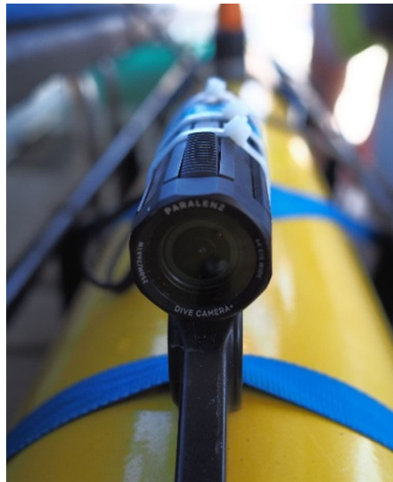
Figure 7. POV camera mounted on the AUV.
