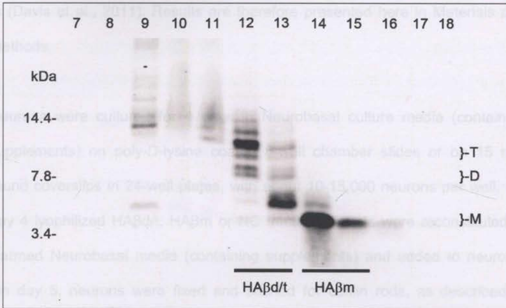
Figure 5.2 Western blot showing fractions of human A\beta monomers ( HA\beta m ) and dimer/trimers ( HA\beta d/t ) purified from 10x concentrated culture medium of 7PA2 cells. Size exclusion chromatography (SEC) fractions 12 and 13 are enriched with dimers (D) and trimers (T) which run between 7.8–14.4 kDa on a 10–20% Tris-Tricine gel. Fractions 14 and 15 are enriched with monomers (M) (4kDa). Source: (Marsden et al., 2011). With thanks to the Bamberg Laboratory, Colorado State University, USA.
