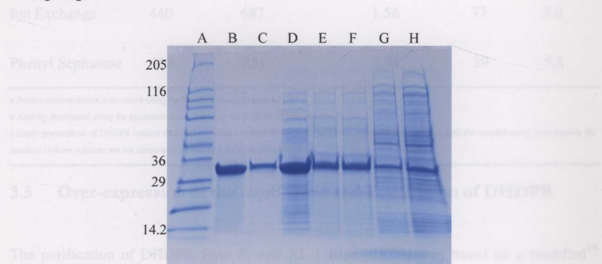
Figure 3.4.1: SDS-PAGE comparison of sample solutions after each DHDPS purification step. LANE A: Sigmamarker, wide molecular weight range, molecular weights of the bands are (from top) 205, 116, 97, 84, 66, 55, 45, 36, 29, 24, 20, 10.2 and 6.5 kDa; LANE B & C: Hi-Trap Q-Sepharose ion exchange fractions; LANES D & E: Phenyl Sepharose; LANE F: Q-Sepharose ion exchange fraction; LANES G & H: Crude cell extract. N.B. duplicate lanes contained different loads.
