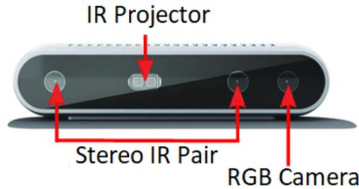
Figure 5.1 Intel RealSense D415 Stereo Depth Camera.
