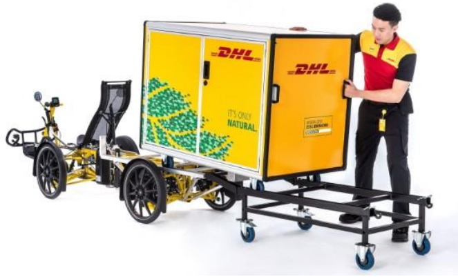
Figure 14 Metre Cube Container loaded onto an E-Cargo Bike (DHL 2019)
