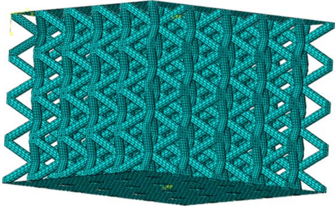
Figure 3.25 Ideal meshed BCC lattice structure created by the GUI
