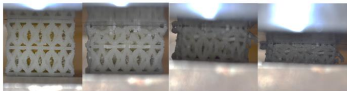
Figure 1.4 Tetrahedron compression test result
