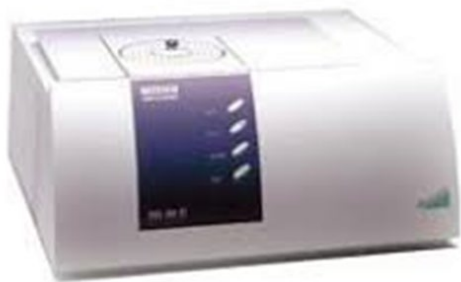
Figure 3.16: (a) Differential scanning calorimetry (DSC) device (Model: Netzsch 204F1), and (b) the operational principle of the DSC technique.
