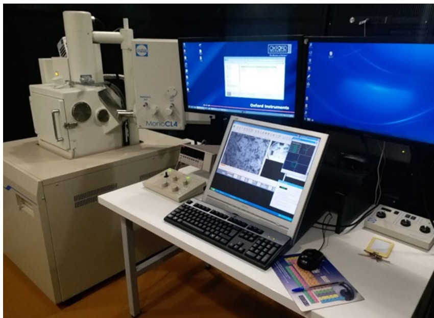
Figure 3.15: Scanning electron microscope (JEOL JSM-6490LV).
