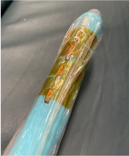
(a) MOSkins placed along the TRUSProbe Tracker. The kapton tape can be seen securing the dosimeters.
