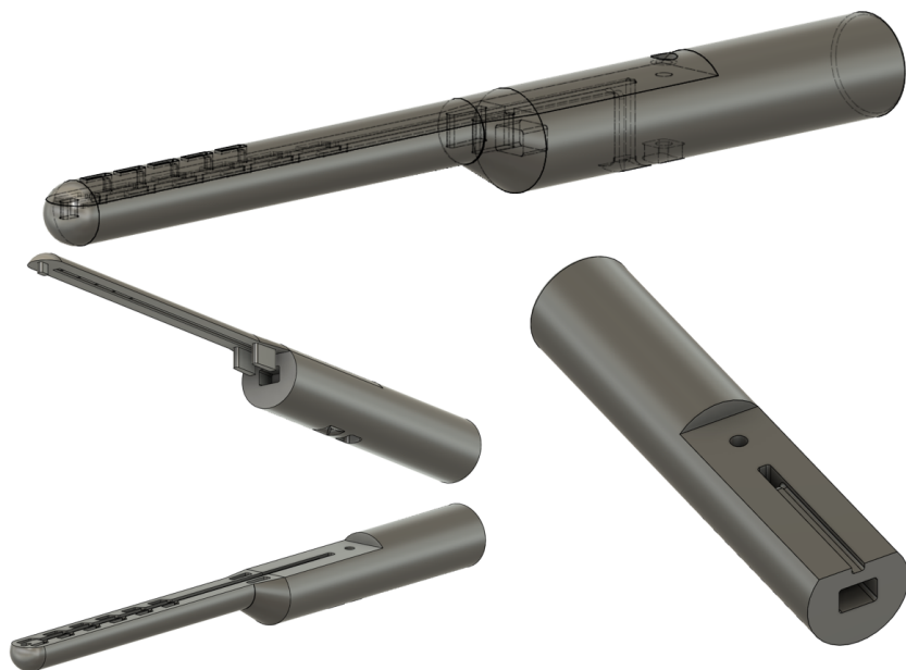
(a) The raw CAD drawings of the TRUSProbe Tracker and the three separate bodies that make up the probe.
