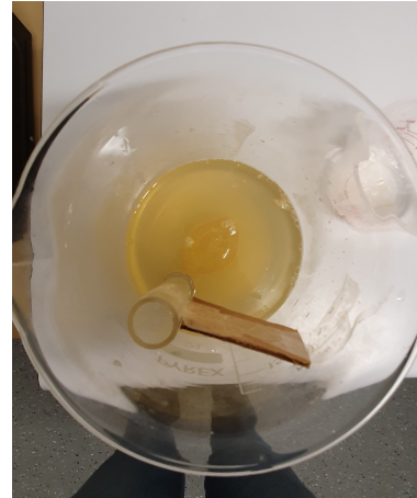
(b) Gel interface US testing. The Gel Prostate insert can be seen surrounded by a different density gel.
