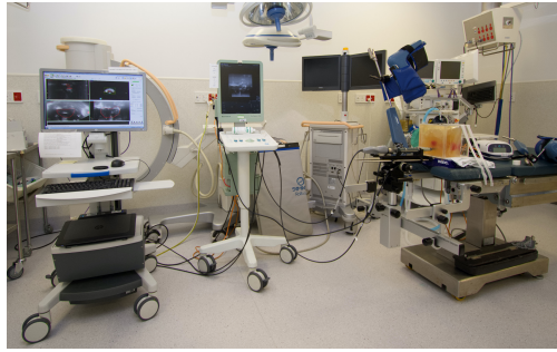
(a) Setup for volumetric study. From left to right; TPS, US system, and TRUS Probe and stepper mount with the E2E phantom secured on the patient couch.
