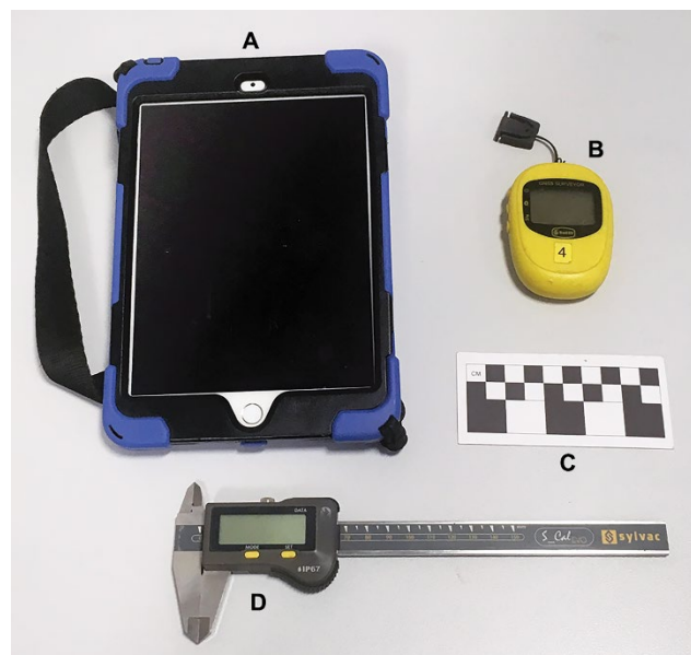
18 Figure 5. Phase 1 archaeological survey kit: A) iPad Mini 4 in rugged case; B) Bad Elf 19 GNSS Surveyor, C) Photo scale; D) Bluetooth digital calipers.
