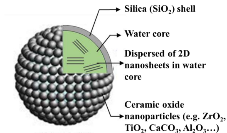
Figure 2-33. The schematic presenting the structure of the proposed colloidal capsule for this research.
