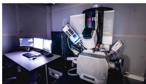
Figure 3-2. Digital image and simplified schematic of dual-beam FIB-SEM instrument 227, 228 .
