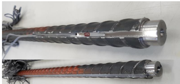
Figure 5: Instrumented and sealed rock bolts
