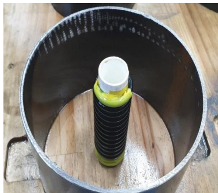
Figure 2: PVC tube used for rifling and hole for installing the bolt
