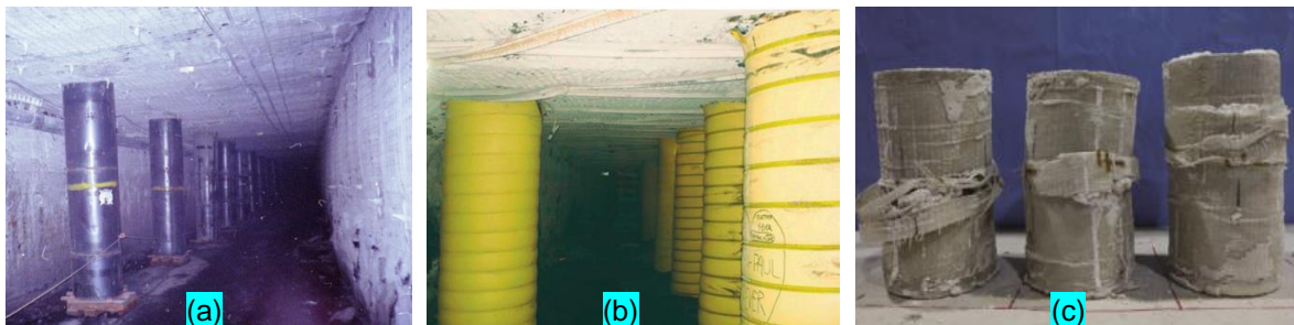
Figure 2: (a) the Can support (Galvin 2016), (b) pumpable standing support (Barczak 2017), and (c) FRP standing support (Zhao et al. 2021)
