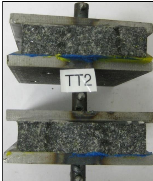
Figure 8: Failed transverse tensile test disc between glued on plates
