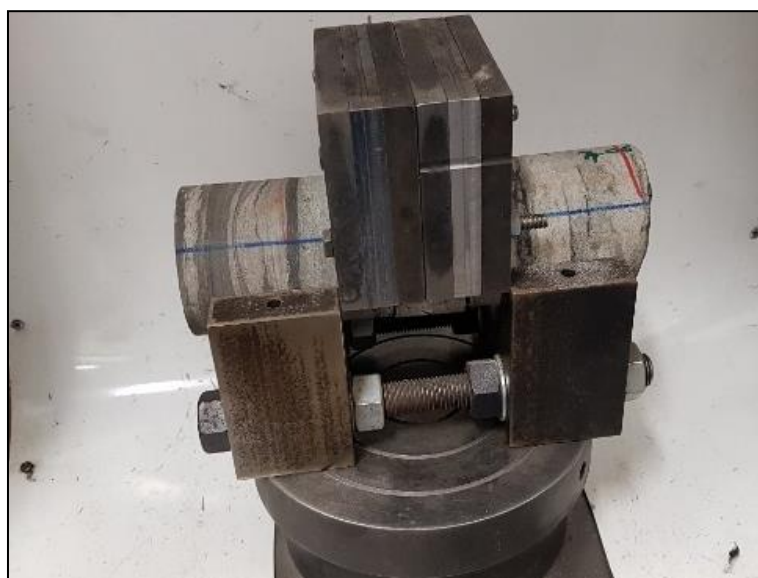
Figure 9: Direct shear test of core
