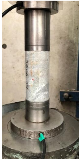
Figure 3: HQ rock sample subject to sonic velocity measurements using (compression) transducers
