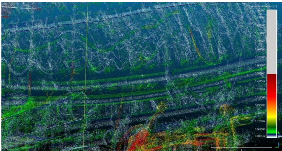
Figure 10: View of the geotechnical station; comparison of changes 576 m x 302 m in front of the longwall
