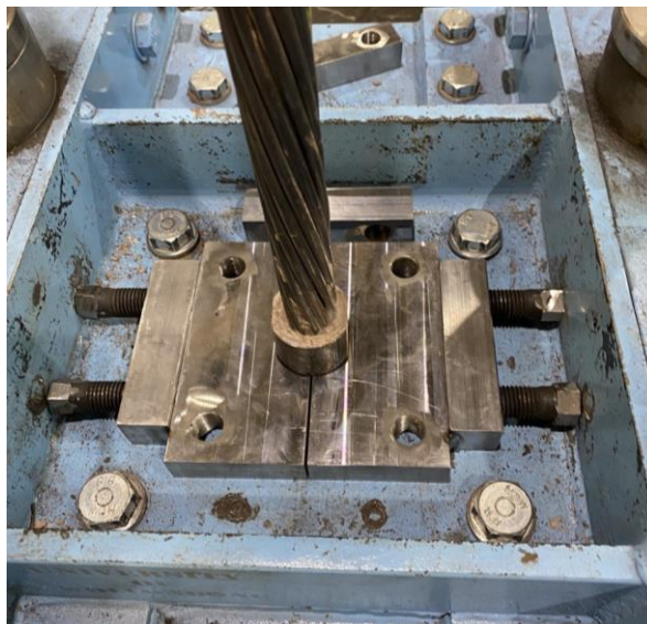
Figure 4: Shorter second embedment length and modified anti-rotation system with minimum friction
