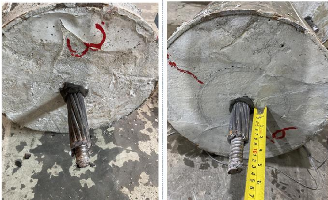
Figure 7: Failure of the bulbed cable bolt in static (Left) and dynamic (Right) pull tests
