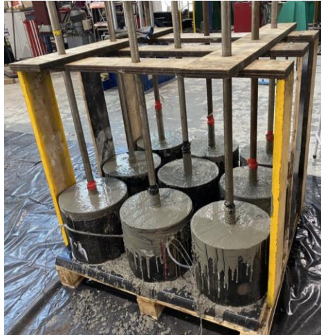
Figure 3: samples cast directly in steel tubes
