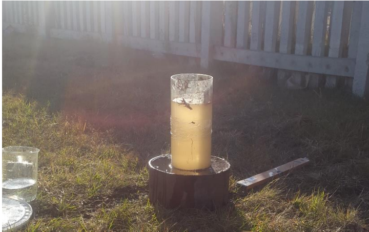
Figure 3-6. Double ring infiltration test setup showing constant head kept in outer ring and observed falling head in inner ring.
