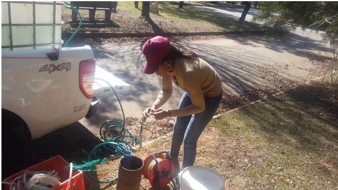
Figure 3-7. Measuring water level in BH3D during a falling head test.
