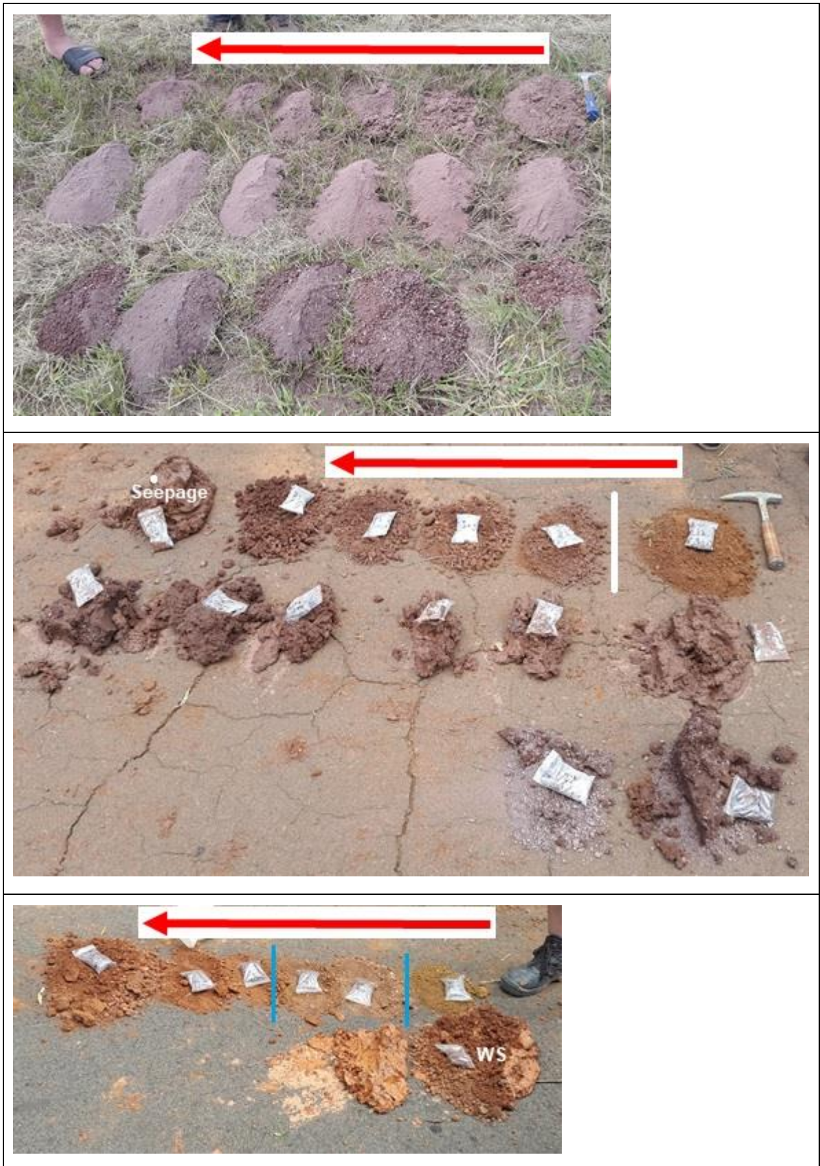
Figure 3-4. Photos showing drill samples laid on the ground. Red arrow shows the direction of increasing depth.
