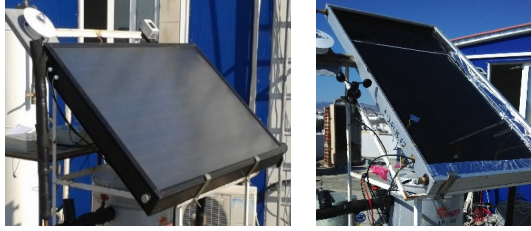
Figure 2: PVT collectors: M1 (left), and M2U (right).
