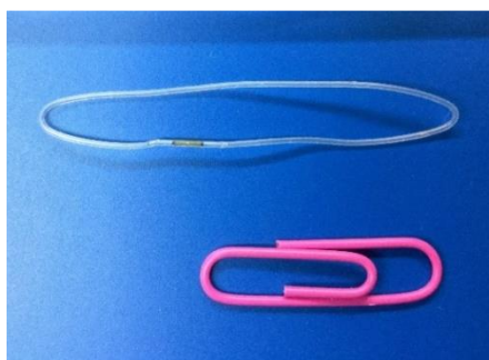
Figure 4.9: PDMS sampling loop; a 10 cm length of a silicone elastomer medical grade tubing joined at the ends by a 1 cm piece of uncoated silica capillary column.
