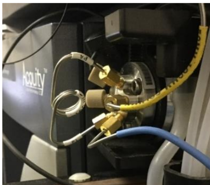
Figure 4.15: UPLC™ system fitted with 100 \mu L sample loop.
