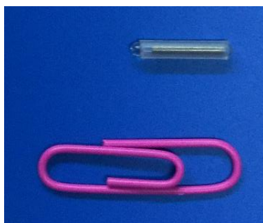
Figure 4.10: Twisters™; magnetic stir bars coated with a volume of PDMS.
