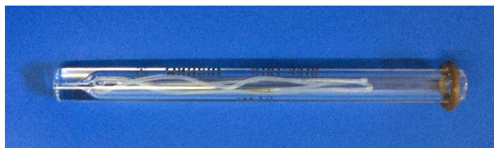
Figure 4.17: GC inlet liner showing inserted PDMS loops.
