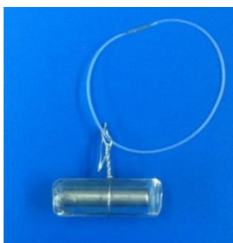
Figure 4.12: PDMS loop secured to a glass stir bar using stainless steel wire.
