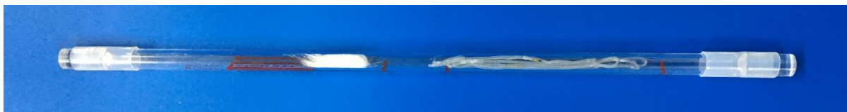
Figure 4.14: Experimental set-up of the thermal desorption tube containing glasswool plug (spiked with 2 µl BSTFA + TMCS (99:1)) and four PDMS loops for the multi-shot derivatisation method.
