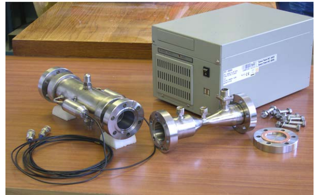
Figure 2 Components of cryogenic two-phase flow-meter for helium and hydrogen: left – RF-sensor of a round cross-section with ID = 38 mm, right – cone ND, background – measuring block based on the 6-slot multichannel industrial computer.
