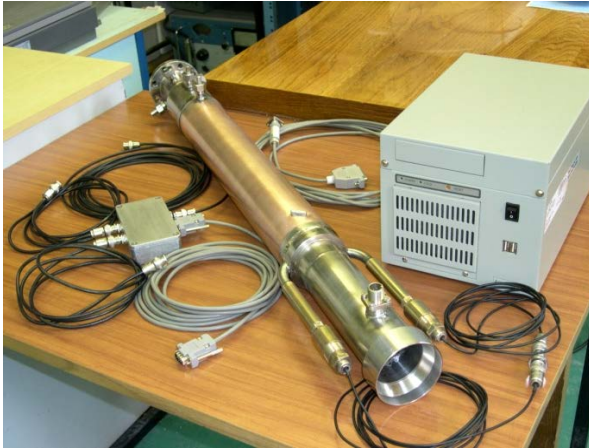
Figure 3 Cryogenic two-phase flow-meter for hydrogen with RF-sensor of annular cross-section (220 mm 2 ) and hemispherical ND.
