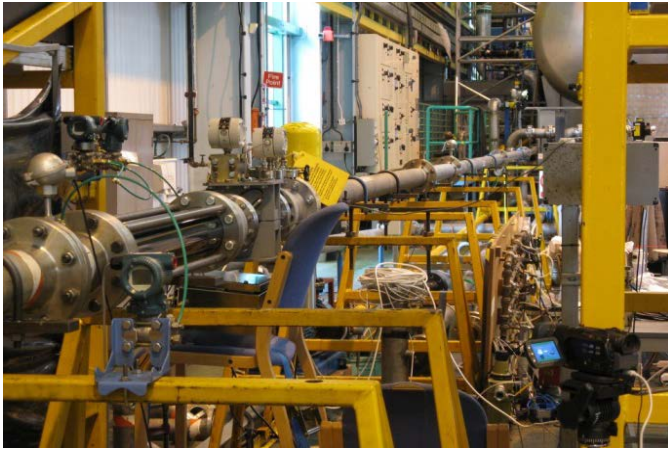
Figure 10 TUV SUD NEL test bench: visual section of ID=102 mm (left), video-camera (right) and investigated flow-meter based on \text{Cs}^{137} GD (yellow color) and cone ND.
