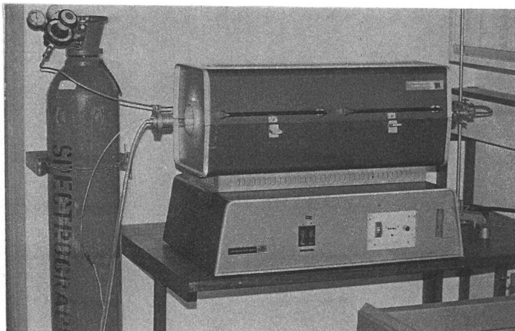
Figure 4.5: Annealing furnace on top of the temperature controller box. The gas inlet on right hand side and gas outlet on left hand side is also visible.
