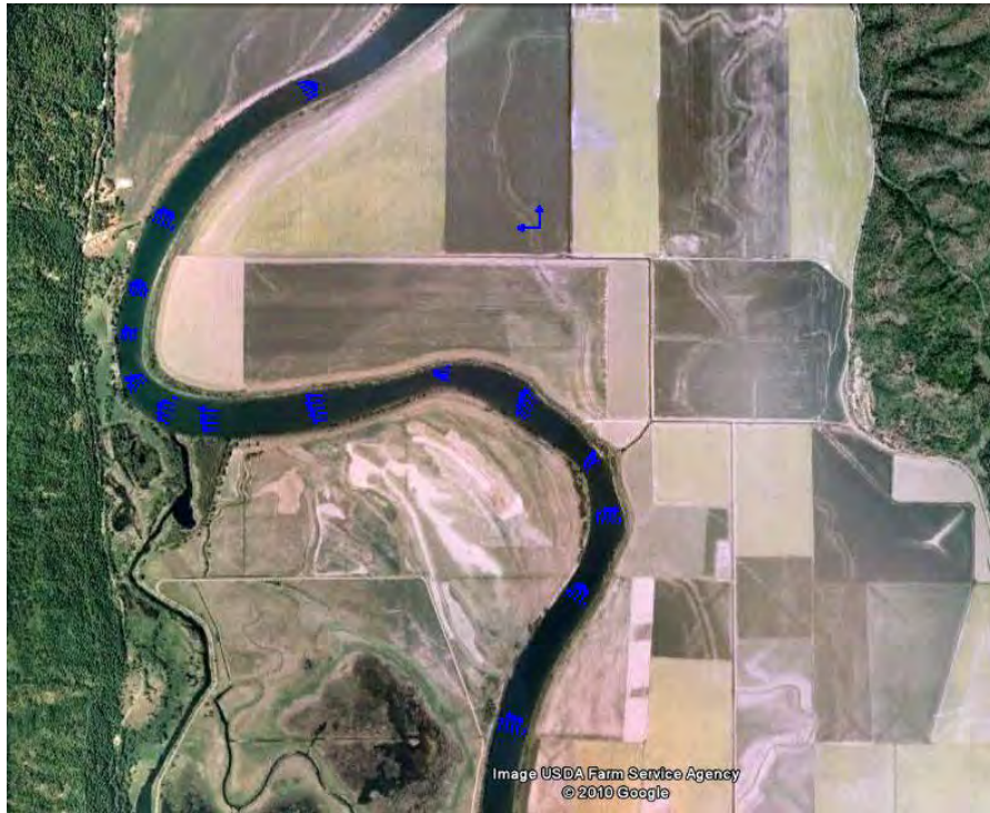
Figure 2. Surface velocity vectors from 10-minute averaged ADCP observation when the USV was station-keeping overlaid on a Google Earth image of the meandering reach of the Kootenai River, ID. 0.5 m/s velocity scale plotted on land.
