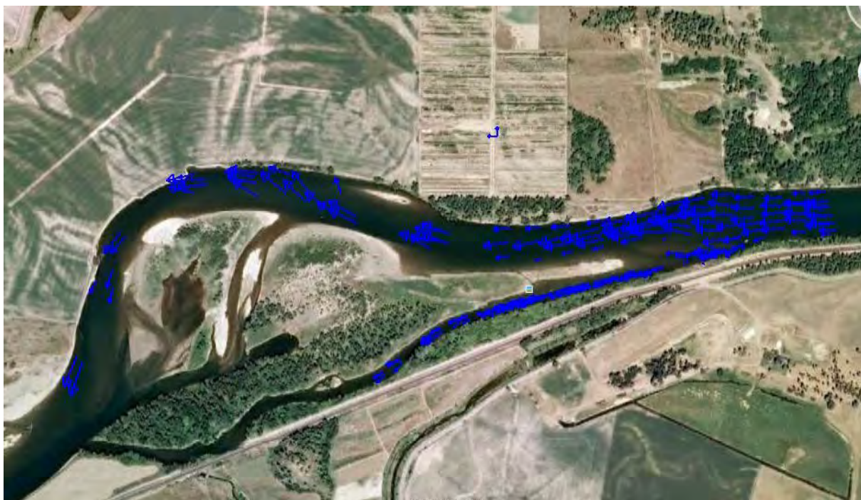
Figure 1. Surface velocity vectors from 15-minute averaged ADCP observation from stationary mini-catamarans overlaid on a Google Earth image of the meandering reach of the Kootenai River, ID. 0.5 m/s velocity scale plotted on the land north of the channel
