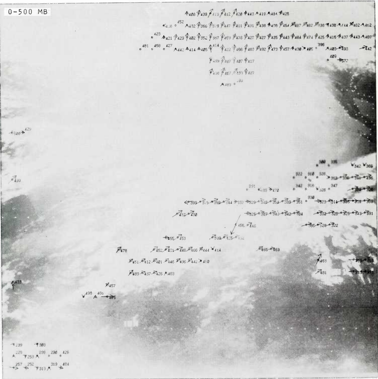
Figure 11a. SAWEGS vectors for upper levels produced by tracking 26 March 1979, 2115/2145 GMT infrared image pair. A 32 by 32 subarea size was used with a 16 pixel overlap of subareas. Vector length is proportional to wind speed; numerals with each observation indicate height in millibars. Quality control has not been applied.
