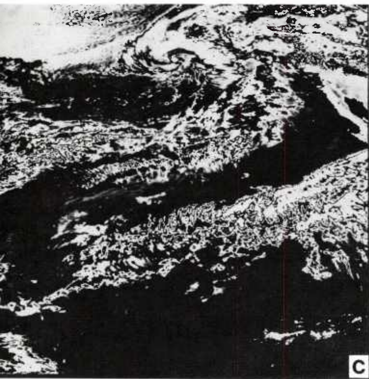
Figure 5. Results of infrared image edge and pattern enhancement. (a) Original unenhanced 8 km resolution infrared image. (b) Result of enhancement based on standard deviation. (c) Result of enhancement based on high order bit truncation.
