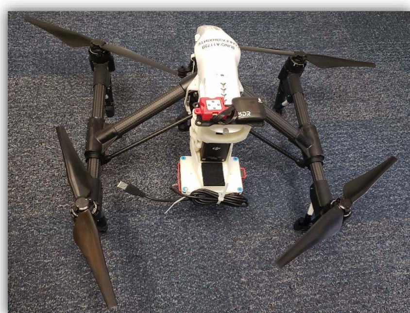
DJI Inspire with Micasense RedEdge-M 5-band camera, currently being used to gather data over water
