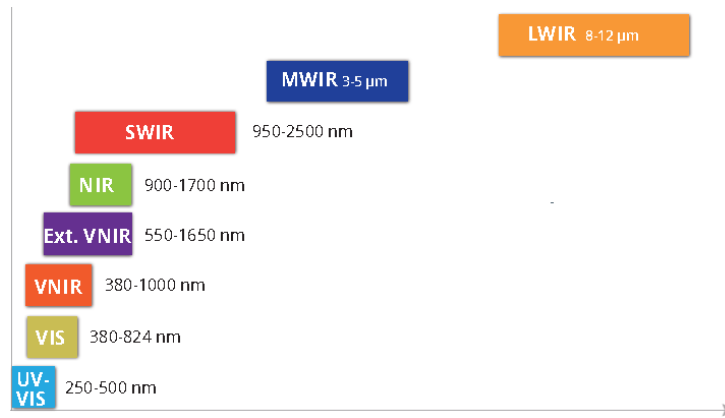
Figure 2. HS ranges for a UAS compatible Micro-Hyperspec sensor family [8].
