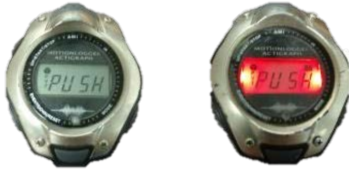
Figure 1. Wrist-worn device (WWD) with the screen backlight feature off (left) and on (right).
