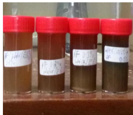
Figure 2. Image of Prepared Palm Kernel Fibre Nanofluid with Di-ionized water and Ethylene Glycol (50:50) as Base Fluid.
