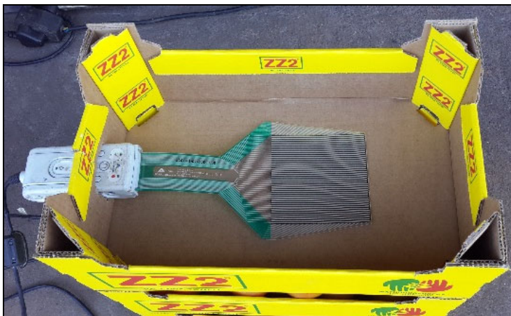
Figure 6 Installation of pressure sensor in small boxes (see online version for colours)
