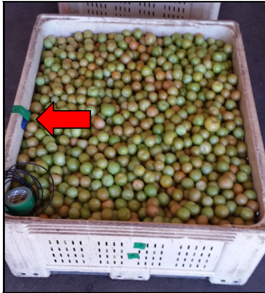
Figure 3 Installation of accelerometers on halfbins (see online version for colours)
