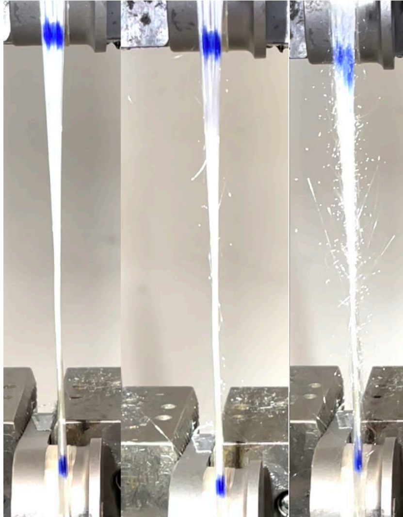
Figure 25. GFB preload (left), as fibers begin to break (middle), and after complete failure (right).
