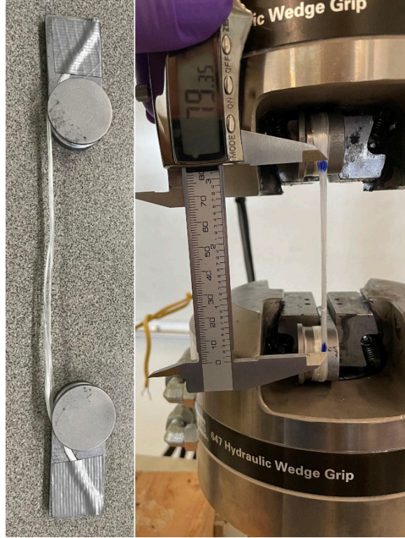
Figure 8. GFB wrapped around the cylindrical adapter before (left) and after (right) being gripped.
