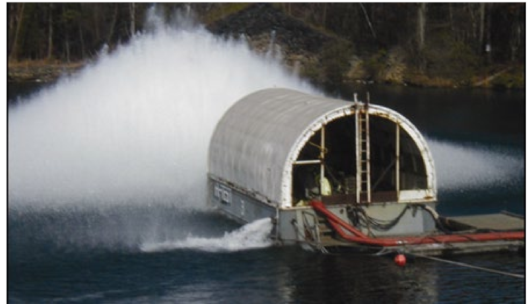
Floating Shock Platform Test for Shipboard Equipment
