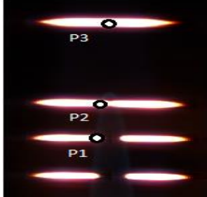
Figure 3 The position of measured points on each glowing SiC fibre; each spot is equivalent to 4mm in length of fibre corresponding to 30 pixels in the image
