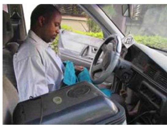
Car battery-powered refrigerator for transportation of samples from the field
