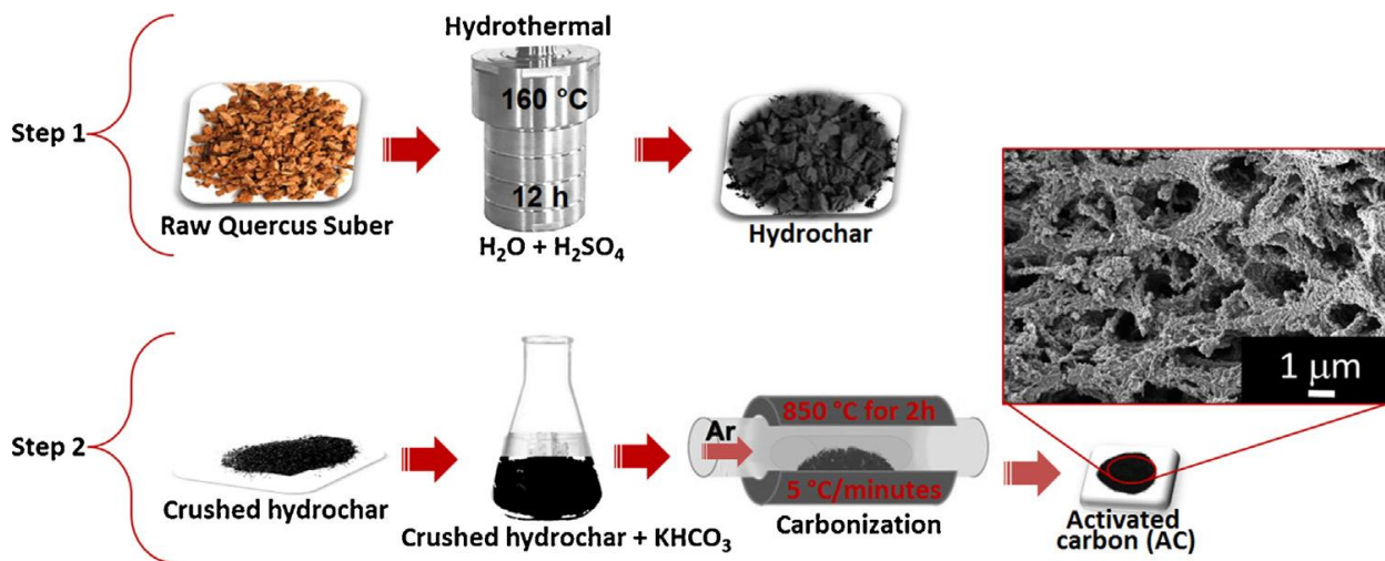
Figure 3.5 Schematic of the Synthesis of activated carbon derived from cork by activation with \text{KHCO}_3
