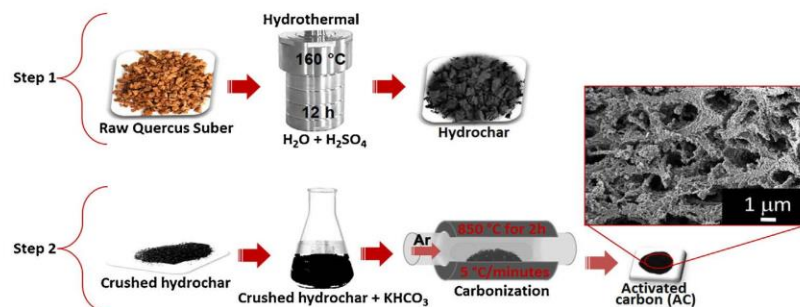
Scheme 2. Schematic of the synthesis route of the activated carbon.
