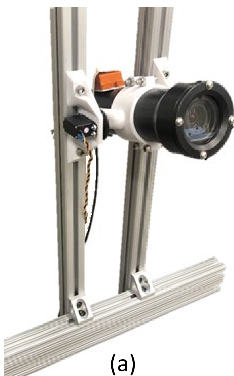
Experimental set-up: (a) 1-DoF rotating camera, (b) sphere used to represent underwater mine.
