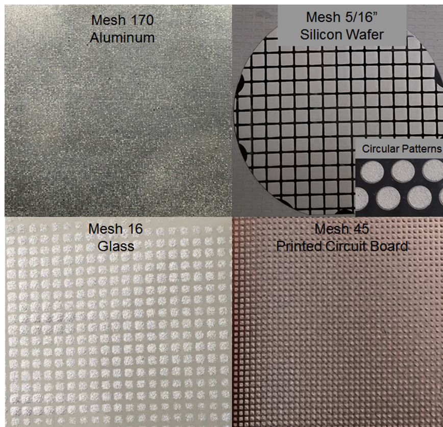
Fig. 2. Two-dimensional features fabricated on aluminum, silicon wafer, glass, and copper foil layer of PCB with cold spray surface patterning technique.
