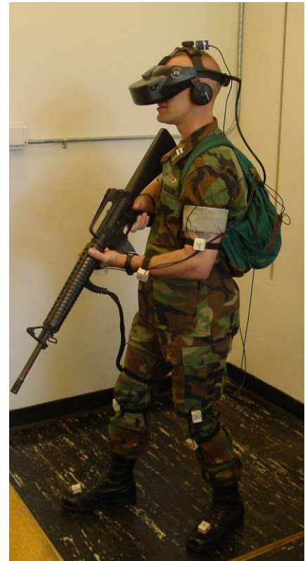
Figure 1: Prototype body tracking system based on inertial/magnetic sensors modules.
