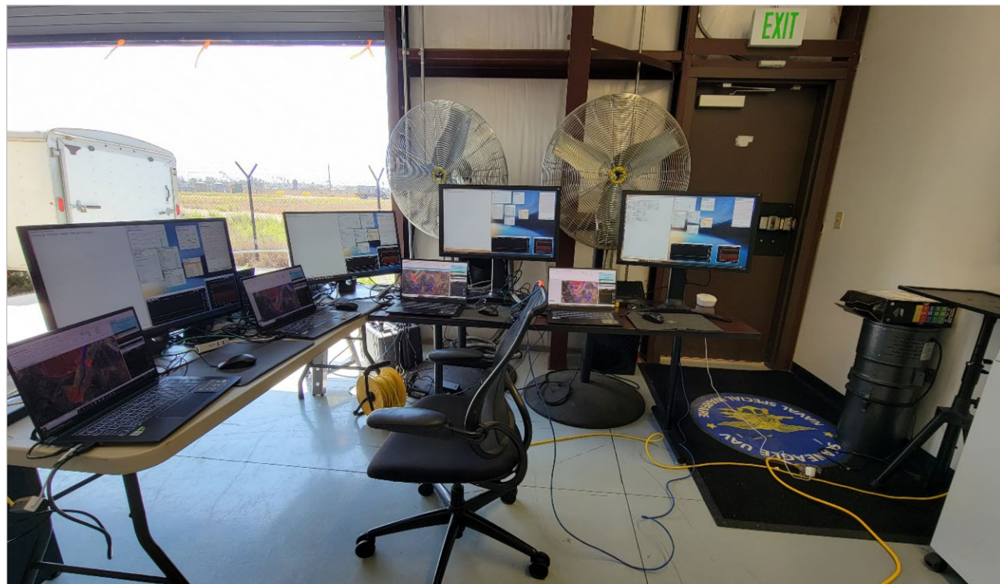
ScanEagle Control Station setup for the control of four ScanEagles
