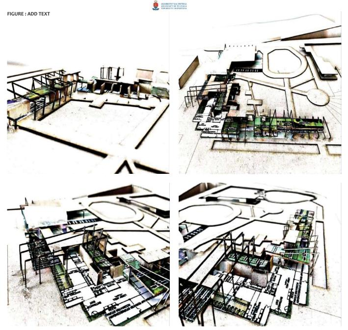
The breaking up of solid forms was the initial urban vision concept which allows for courtyard recreational areas as well as more green niches that are situated be The span of the portal frames ranged to up to 12m span and therefore a steel coloumn will be added at every 6m intervals in order to allow for manual assemble. This will enable future expansion to be easier. ween masses.
