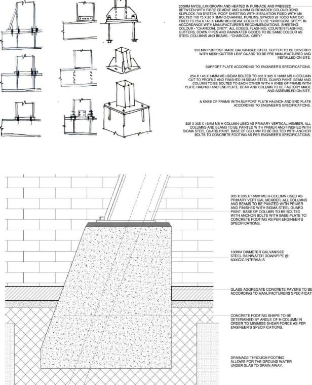
305 X 305 X 16MM MS H-COLUMN USED AS PRIMARY VERTICAL MEMBER. ALL COLUMNS AND BEAMS TO BE PAINTED WITH PRIMER AND FINISHED WITH SIGMA STEEL GUARD PAINT. BASE OF COLUMN TO BE BOLTED WITH ANCHOR BOLTS WITH BASE PLATE TO CONGRETE FOOTING AS PER ENGINEER'S SPECIFICATIONS.
