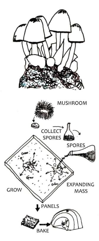
FIG 6.22 : How to make mycelium insulation or brick (Author 2019)
