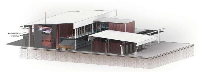
Fig. 7.15: Furnace and water heating sectional perspective (Author 2019)
