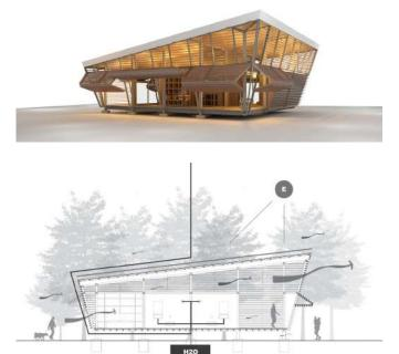
The structure is compiled of an inclined exterior façade which limits the amount of impact precipitation and sunlight has, thus limiting water splashing on the surface as well as overheating. The vertical structural columns carry of internal load therefore allowing the façade panels to be adaptable in order to regulate air flow through the building as well as to regulate views as desired (Ott 2019).
