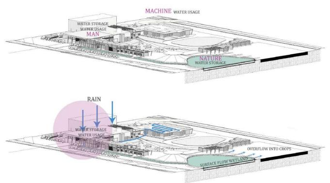
Fig. 7.14: Water harvesting axonometric (Author 2019)
