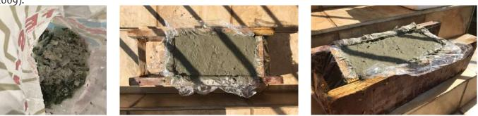
FIG 6.12: Making of crushed glass and concrete blocks (Made by Author
