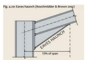
According to Koschmidder and Brown (2012), the size of the haunch is required to be 10% of the portal span and typically is defined from the tapers section of the portal span to the centre-line of the column as illustrated below.
