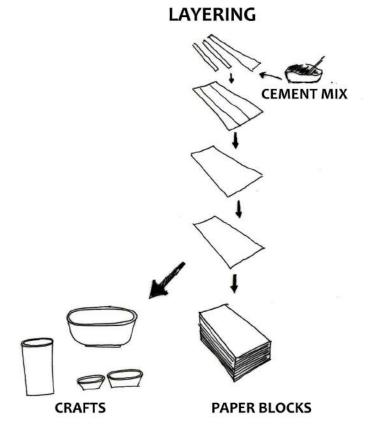
Fig. 6.6: The layering process of paper bricks (Author 2019)
