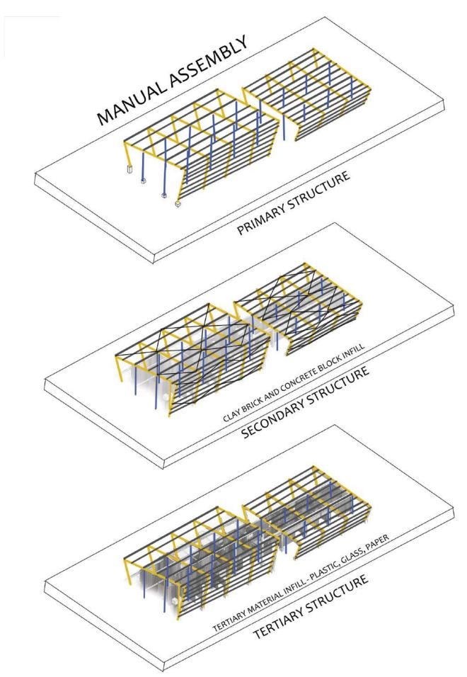
Fig. 7.7: Structure diagram demonstrating the primary, secondary and tertiary structure (Author 2019)
