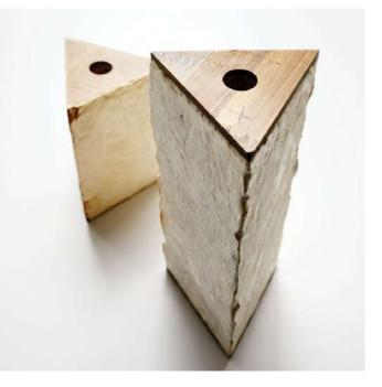
A self-supporting structure that has been grown by engineer Philippe Block and architect Dirk Hebel has proven the potential that mushroom mycelim has in the architecture and design industry (Aouf, 2018). FIG 6.23, 6.24, 6.25, 6.26 : How to make mycelium self-supporting structure (Aouf, 2018).
