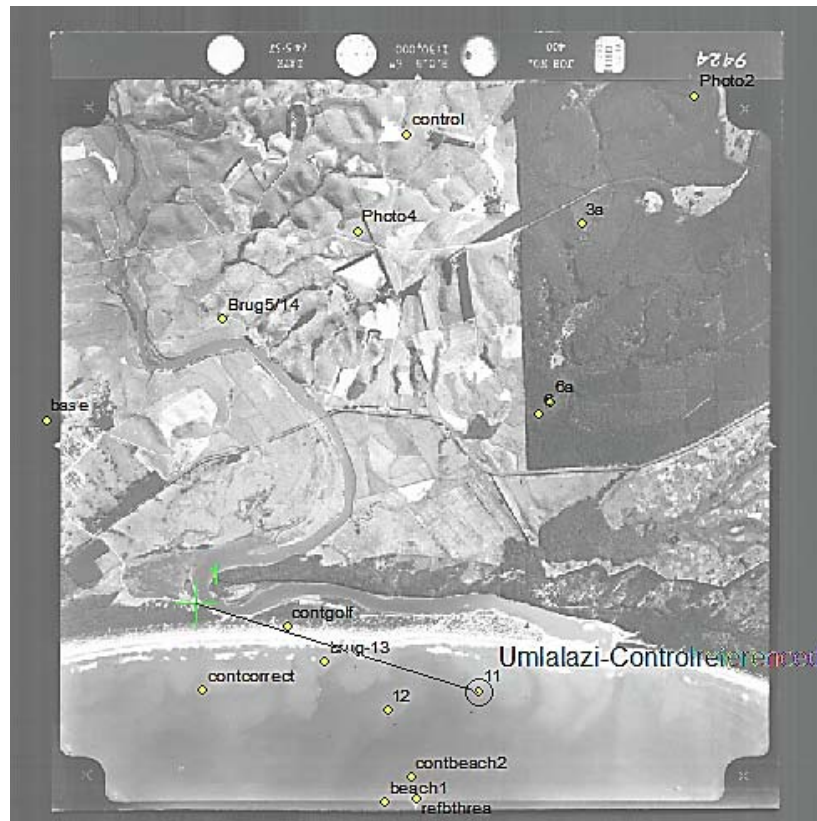
Figure 4.16: The image target with a transparency of 40% is ready to be oriented. The yellow points are the control points. Point 1 on the ground is joined up with Control 11. After another coordinate orientation the photograph will already be provisionally oriented.
