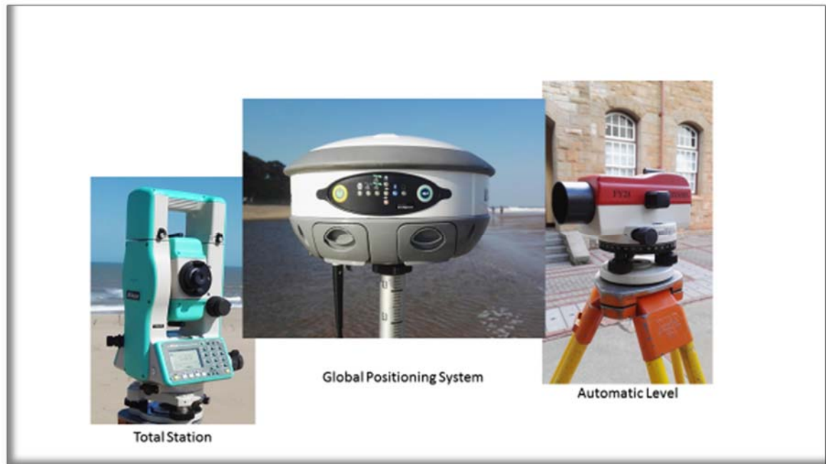
Figure 2.13: Different instruments that surveyors use: (from left to right) a total station, a GPS and an automatic level (instruments photographed courtesy of the University of Pretoria).
