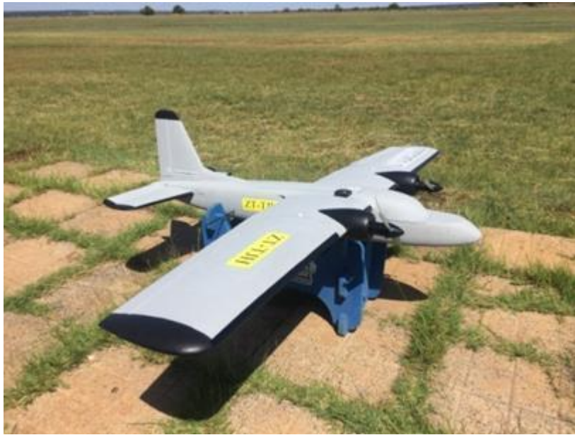
Figure 7: Customized fixed wing UAV that was used to autonomously capture single geotagged images.
