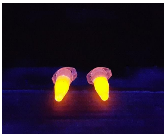
Figure 8. Synthesized polymers with template removed under UV irradiation with an excitation wavelength 365 nm; MIP@QDs (left), NIP@QDs (right).
