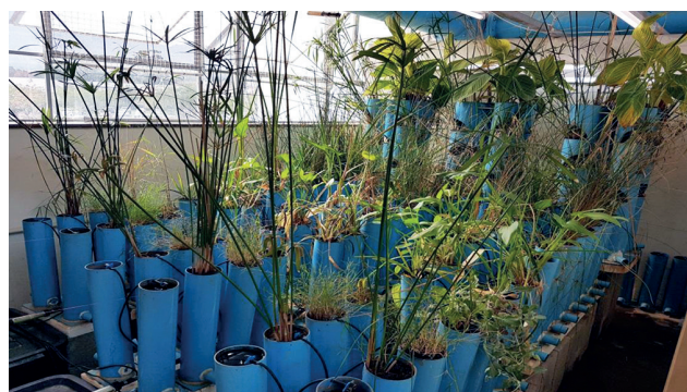
Figure 2. Experimental layout of the constructed laboratory phytoremediation system
